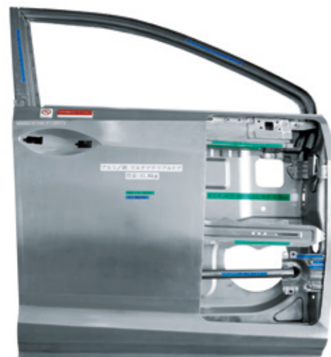
Multi-material door structure originally developed by the KOBELCO Group (prototype)
