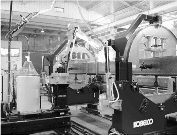
Fig.1 Structural steel large assembly welding robot system
