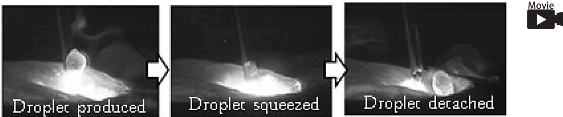
Fig.6 Metal droplet transfer by new process
