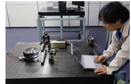
【Testing the machine that automatically measures the appearance (360° image) of molds】
