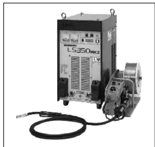
Fig. 1-2 A set of welding power source, wire feeder, and welding torch (Source: a brochure of Kobe Steel, Ltd.)
