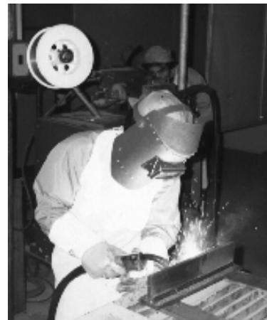
Fig. 2-9 Proper positioning of the welding torch in horizontal-fillet welding
