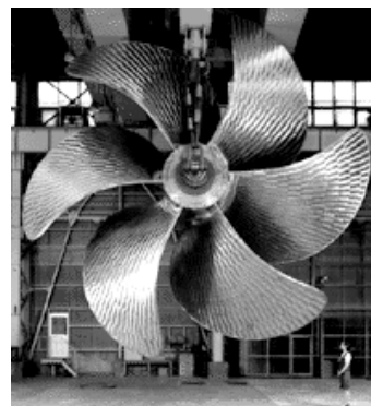
Photo 1.3 Marine propellers are typical applications for copper alloy castings (Photo courtesy of Nakashima Propeller Co., Ltd., Japan)
