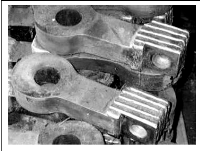
Photo 7.1 — Sugar mill hammerheads hard-faced with a stringer pattern providing harder weld reinforcement on ductile underlayers for better wear resistance
