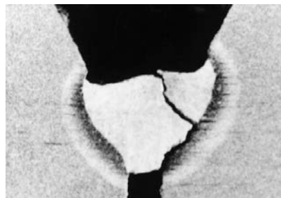
(F) Root crack
