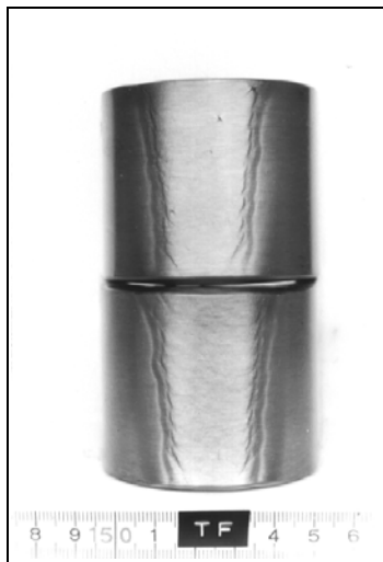
Fig. 6.4 — Side bend specimens after test
