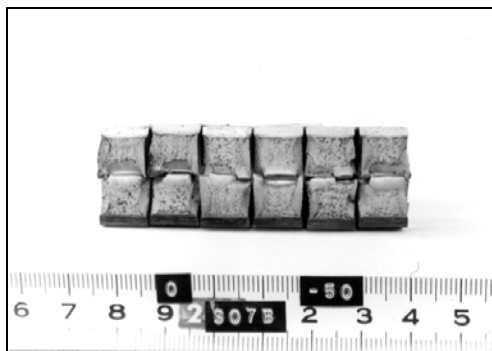
Fig. 6.6 — Fracture surfaces of Charpy impact test specimens after test
