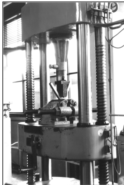
Fig. 6.5 — A bend test machine for roller bend test
