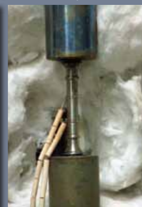
Figure 2: Creep test piece set up
