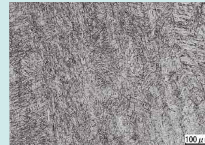
Photo 1: Microstructure of final pass deposited metal (PWHT: 779°C x 8.0 hour)
