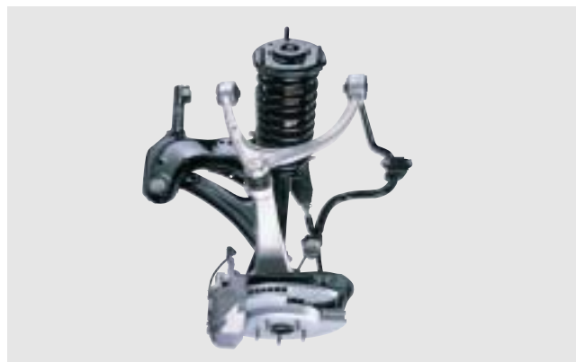
Aluminum forgings in suspension systems contribute to lighter cars. Demand for these and other aluminum products are expected to grow.
