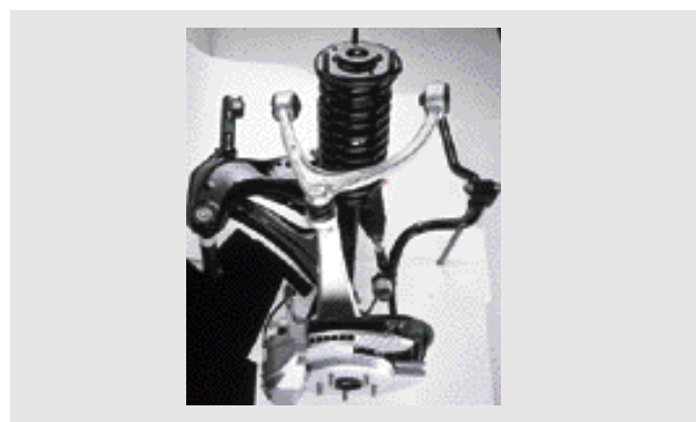
Aluminum forgings in suspension systems contribute to lighter cars. Demand for these and other aluminum products are expected to grow.
