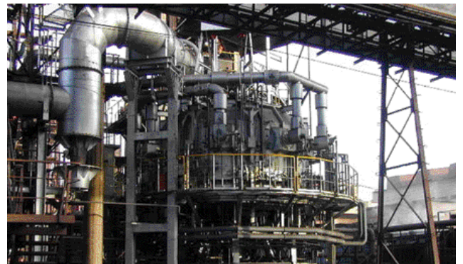
The ITmk3® Process produces high quality iron nuggets, while emitting 20% less carbon dioxide than blast furnace operations. The photo shows the bench-scale plant at the Kakogawa Works.
