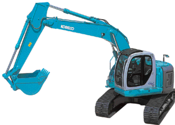
The 200SR is one in a series of excavators with zero tail swing. We pioneered this space-saving feature now found in both mini excavators and excavators.
