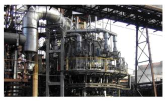
The ITmk3\* Process produces high quality iron nuggets, while emitting 20% less carbon dioxide than blast furnace operations. The photo shows the bench-scale plant at the Kakogawa Works.
