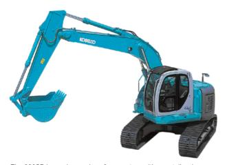
The 200SR is one in a series of excavators with zero tail swing. We pioneered this space-saving features now found in both mini excavators and excavators.
