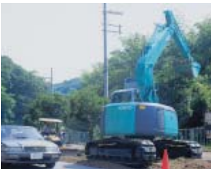
The SK135SR is one in a series of excavators with zero tail swing. We pioneered this space-saving feature now found in both mini excavators and excavators.
