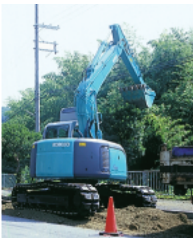
The SK135SR is one in a series of excavators with zero tail swing. We pioneered this space-saving feature now found in both mini excavators and excavators.
