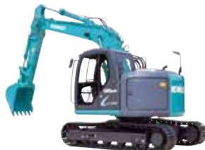
Zero tail swing excavator
