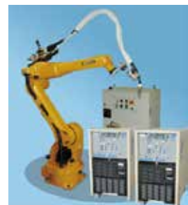
High deposition welding process using two parallel-connected welding power sources
