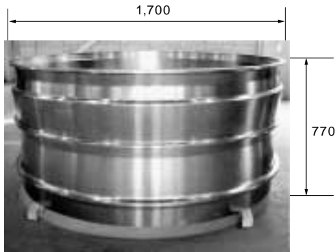
Photo 1 Shipment shape of fan case front
