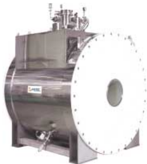
Photo 3 Outside view of 7T/400SS superconducting magnet for animal MRI
