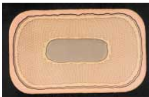
Photo 1 Cross-section of Ta reinforced Nb 3 Sn superconductor
