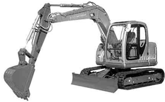
Photo 1 Hybrid excavator (Monitor machine)
