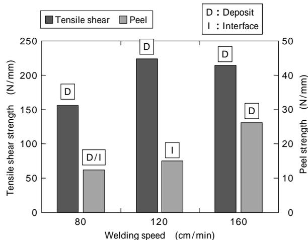
Fig. 6 Relation between welding speed and joints strength
