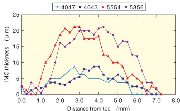
Fig. 5 Distribution of IMC thickness (MIG brazing)
