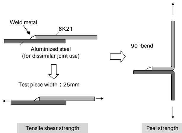
Fig. 3 Evaluation method (tensile shear & peel)
