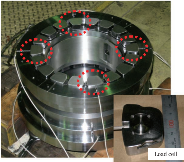
Fig. 10 Thrust bearing with load cell (for measurement of gas thrust force)
