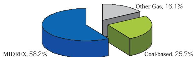
Fig. 2 World-wide direct reduced iron production process in 2008
