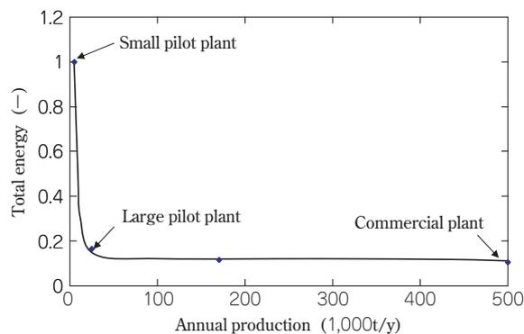
Fig.10 Production size vs. energy consumption
