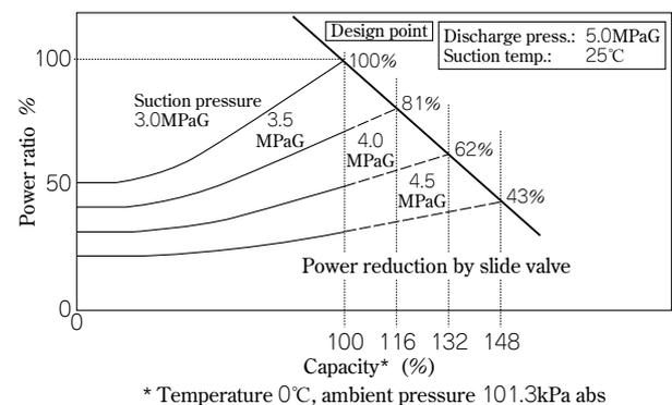
Fig. 8 Typical load characteristics of an oil-flooded compressor
