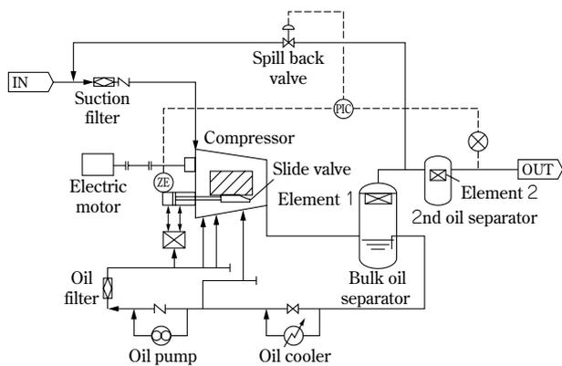
Fig. 4 Schematic diagram of oil-flooded screw compressor
