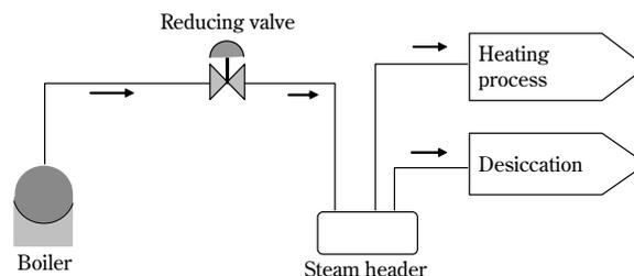
Fig. 1 General process flow in small-sized steam plant
