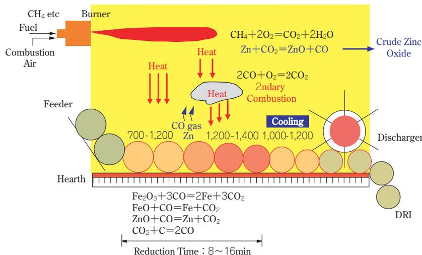
Fig. 2 Schematic drawing of reduction in FASTMET furnace
