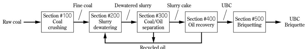
**Fig. 3** Block flow diagram of UBC process
