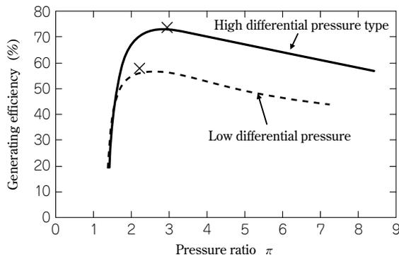
**Fig.14** Relationship between pressure ratio and generating efficiency
