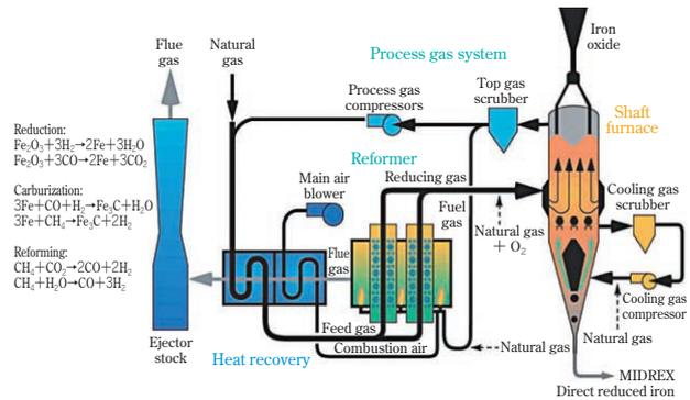
Fig. 3 MIDREX process flow sheet
