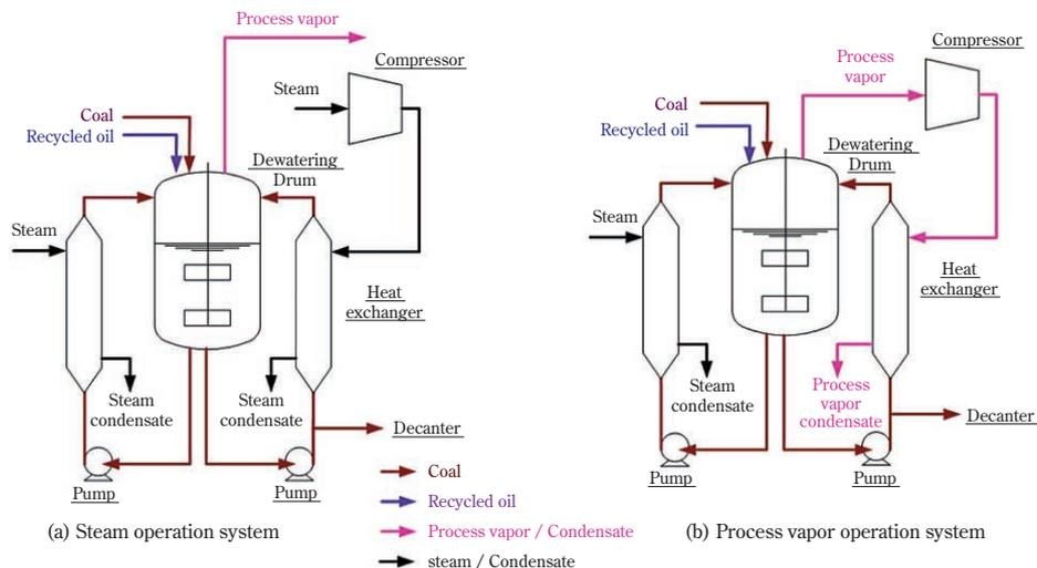
Fig. 8 Diagram of process flow around compressor
