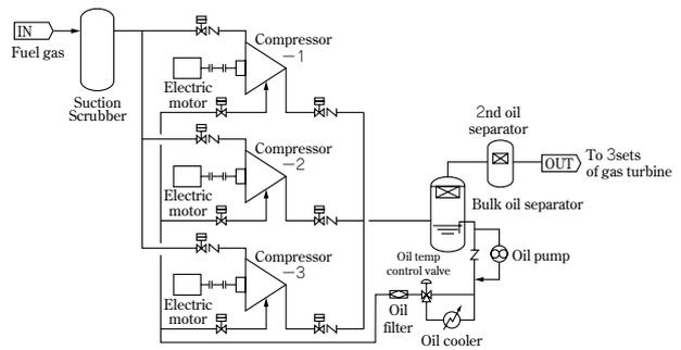
Fig.10 Oil-flooded screw compressor system (case 2)
