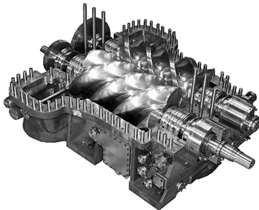
Fig. 2 Horizontally split compressor casing
