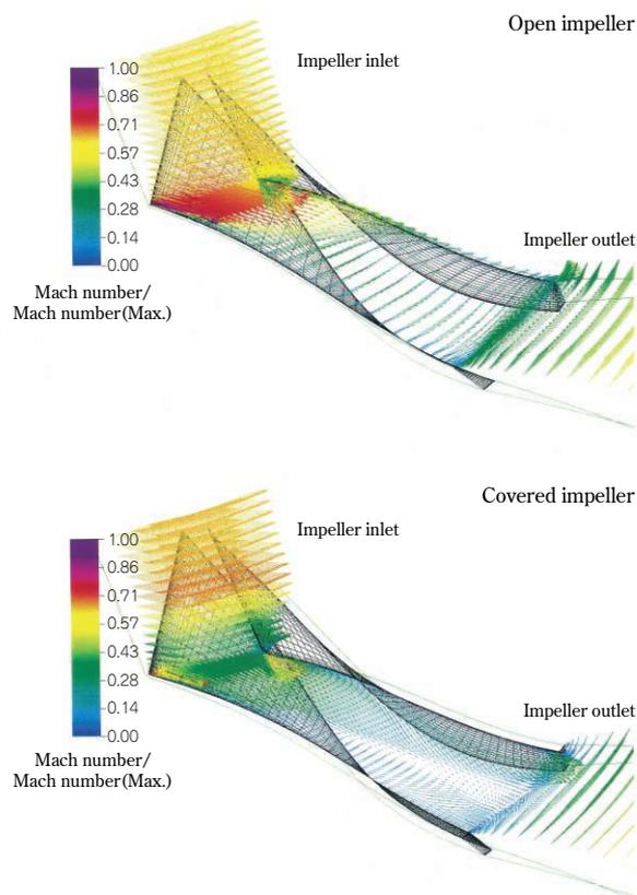
Fig. 4 Example of flow analysis of impeller
