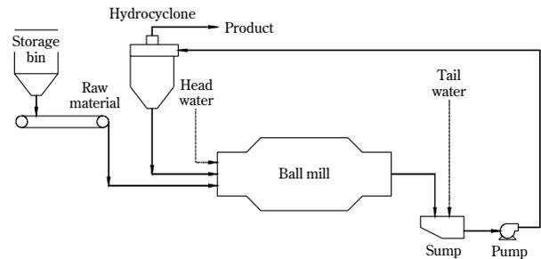
**Fig. 3** Flow of closed circuit wet-grinding system
