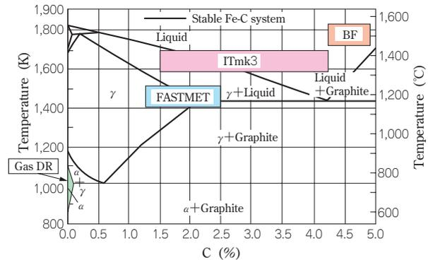
Fig. 1 Operational region of ironmaking processes
