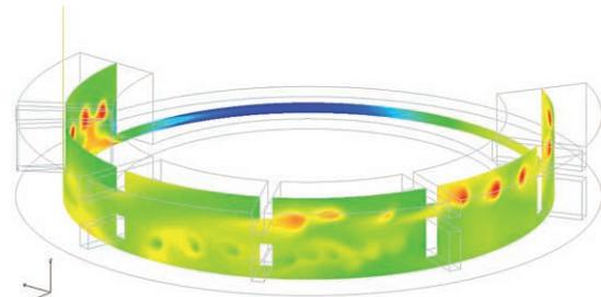
Fig. 7 CFD analysis result for rotary hearth furnace
