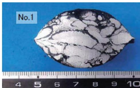
Fig. 6 Sectional view of HBI
