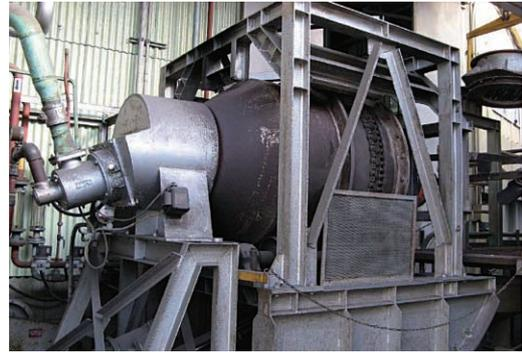
Fig.16 Photograph of batch type kiln
