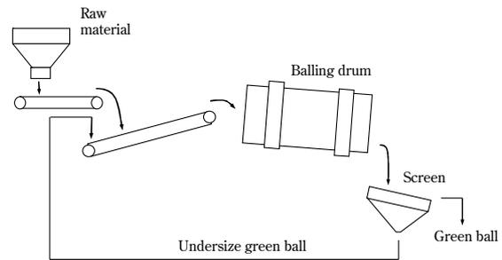
**Fig. 5** Flow of balling drum
