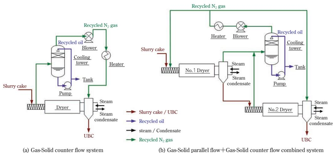
Fig. 9 Diagram of process flow around dryer
