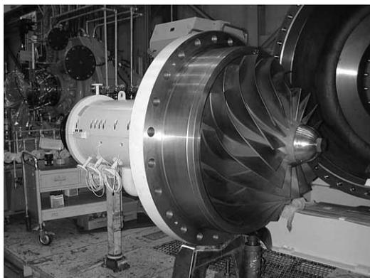
Fig. 6 Example of dismantling of rotor assembly
