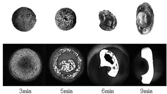
Fig. 5 ITmk3 reaction mechanism
