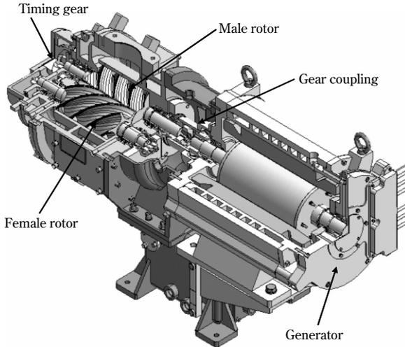
Fig. 5 Main structure of micro steam energy generator
