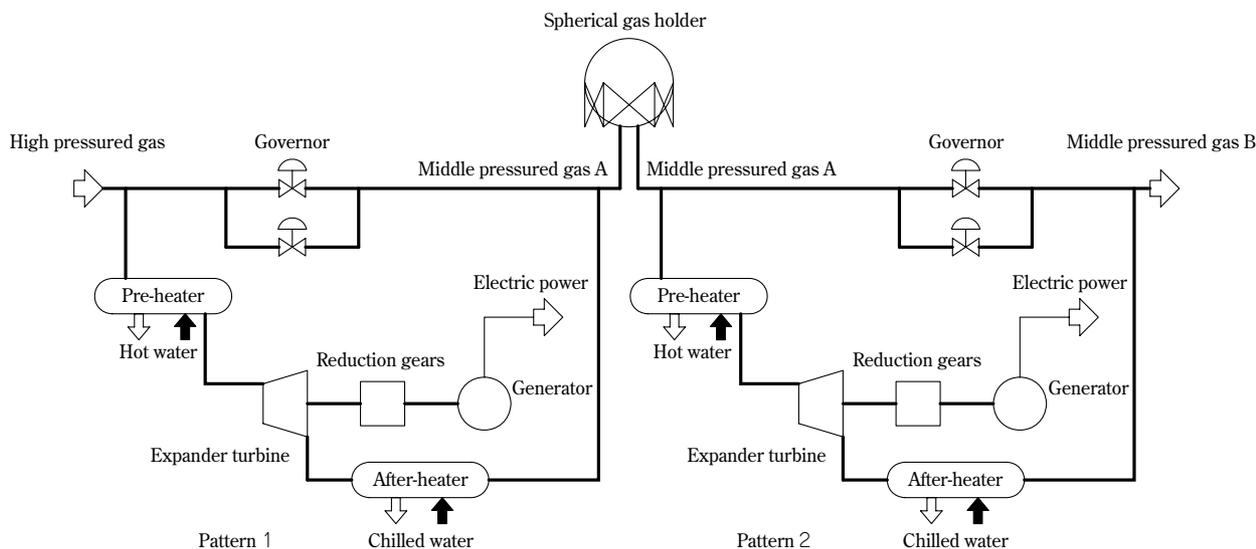
Fig. 2 System flow of gas energy recovery system
