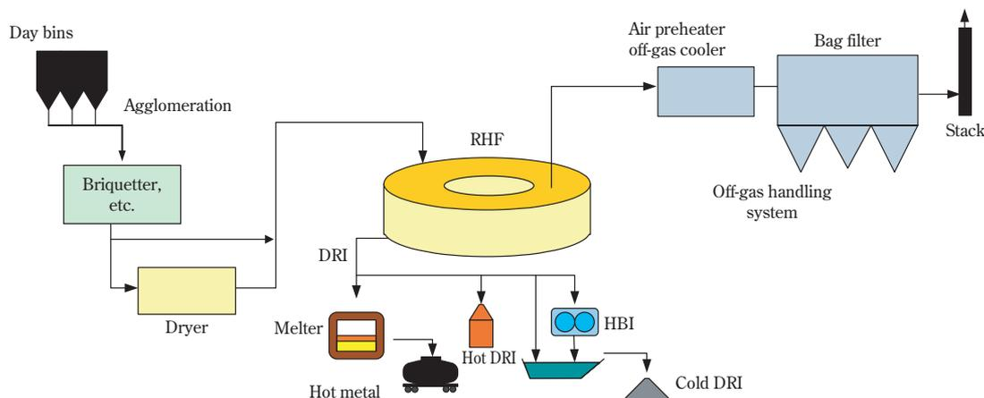
Fig. 3 Process flow sheet for FASTMET
