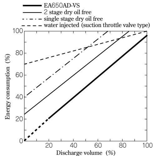
Fig. 6 Performance comparison (37kW class oil-free compressor)
