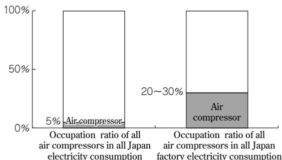
Fig. 1 Electricity consumption ratio of compressor<sup>1)</sup>
