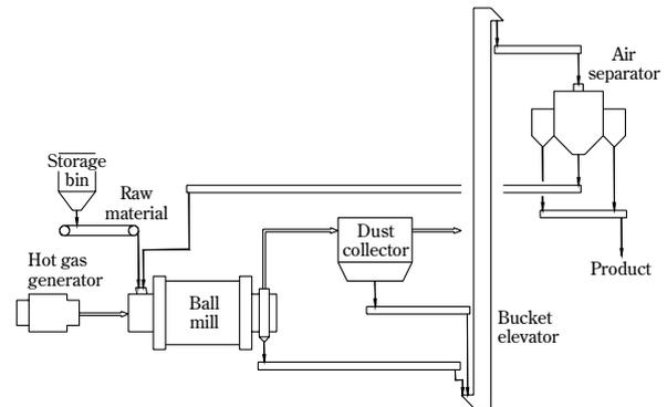
**Fig. 4** Flow of closed circuit dry-grinding system
