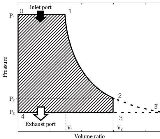
Fig. 7 Indicator diagram
