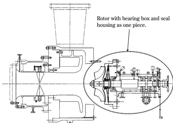
Fig. 5 Dismantling of rotor assembly from compressor casing
