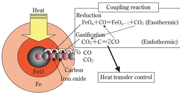
Fig. 2 Reduction mechanism of carbon composite pellet
