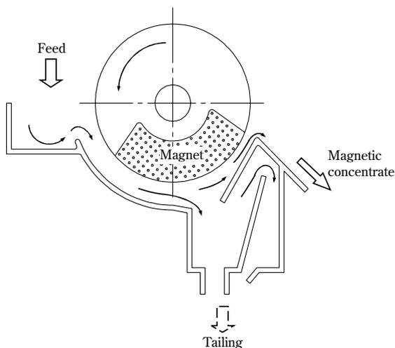
**Fig. 2** Magnetic separator
