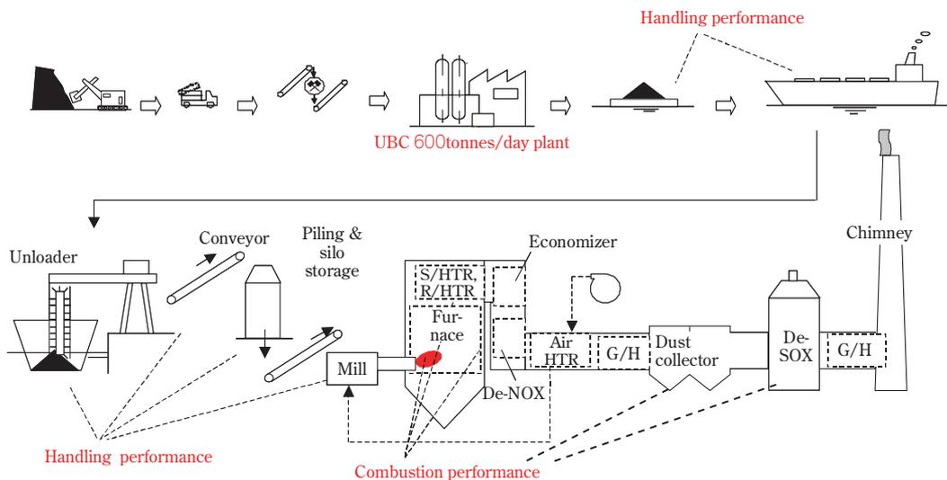
Fig. 6 Items of technical evaluation in combustion test
