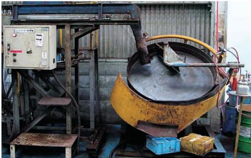
Fig.14 Photograph of balling disc
