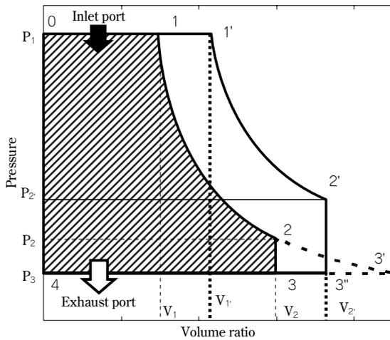
Fig. 9 Indicator diagram-1
