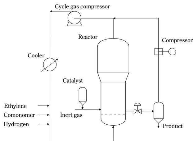
Fig. 1 Typical polyolefin plant process<sup>2)</sup>
