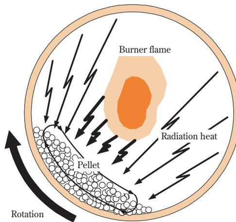
Fig.12 Cross sectional sketch of rotary kiln
