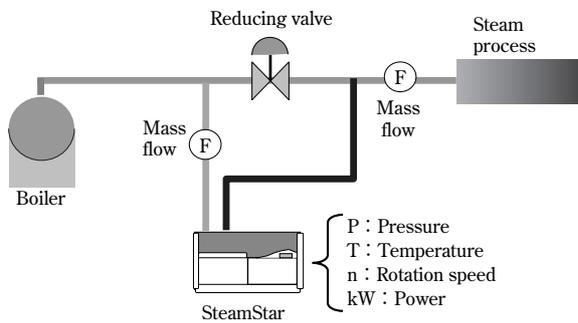
**Fig.11** Flow chart of test facility
