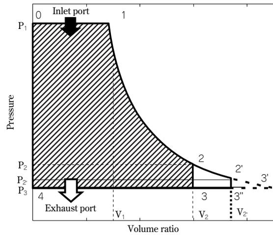
Fig.10 Indicator diagram-2
