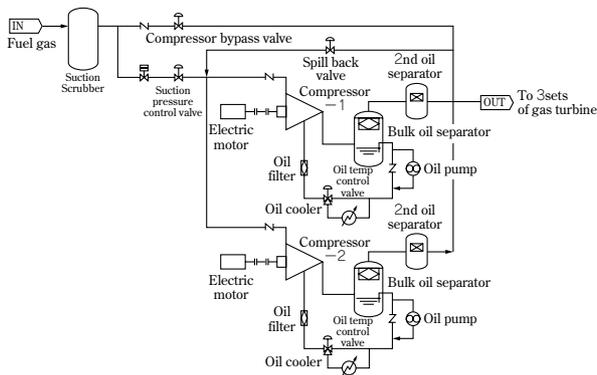
Fig. 9 Oil-flooded screw compressor system (case 1)
