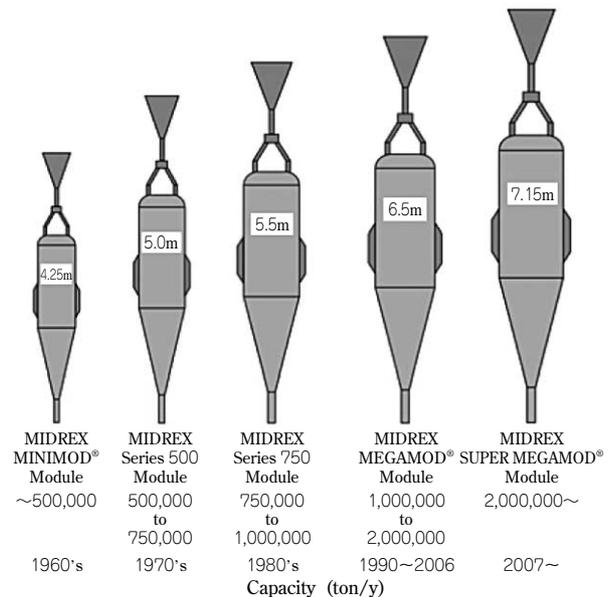
Fig. 7 Changes in shaft furnace diameter and annual production
