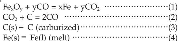
Reactions (1) and (2) occur in the FASTMET process. In the ITmk3 process, there are the additional reactions (3) and (4), which separate metallic iron from slag.
