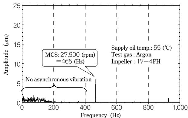
Fig. 9 Test result of SFD bearing
