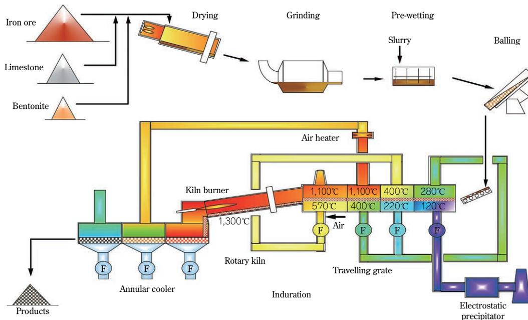
Fig. 7 Typical flow of KOBELCO pelletizing plant
