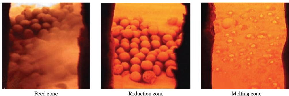
Fig. 9 Inside views of RHF at small pilot plant in Kakogawa Works
