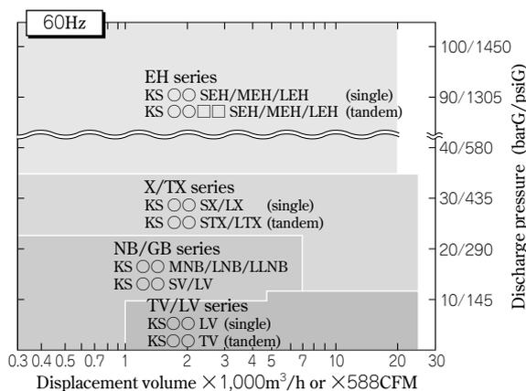
Fig. 1 Range chart for KOBELCO EH series
