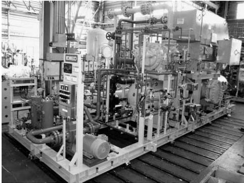
Fig. 7 Screw compressor for gas turbine fuel gas
