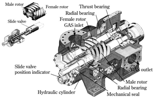
Fig. 2 Construction of 100 barG oil-flooded screw compressor
