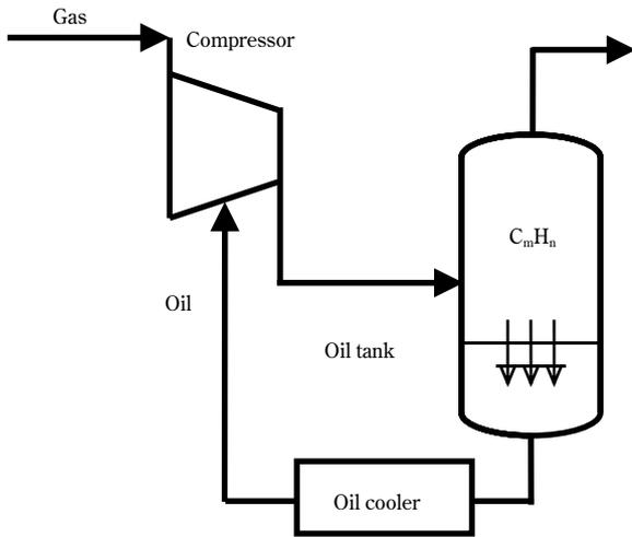
Fig. 9 Flow diagram of an oil-flooded screw compressor
