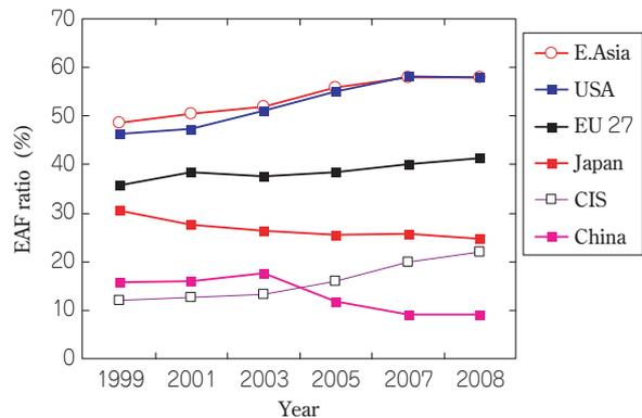
Fig. 7 EAF ratio of crude steel production
