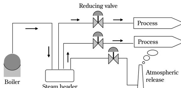
Fig. 2 Process flow in small-sized steam plant with excess steam
