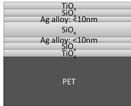
Fig.10 Cross-sectional view of heat reflective film
