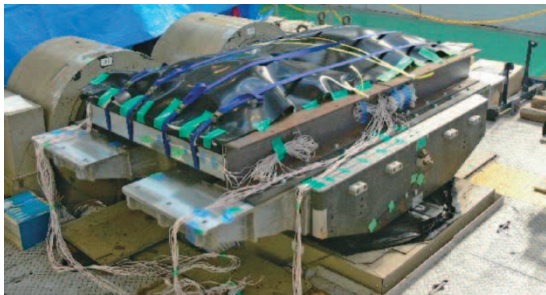
Fig. 8 Load fatigue test of microperforated panel
