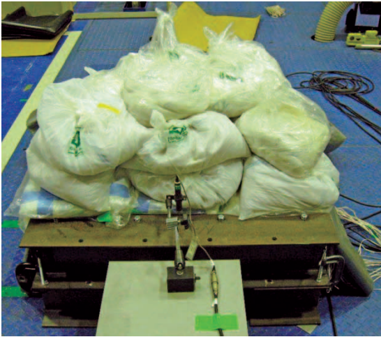
Fig. 7 Static load test of microperforated panel
