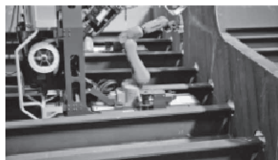
Fig. 3 Small size welding robot
