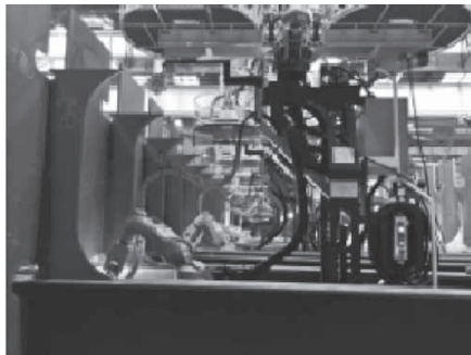
Fig. 4 Application of welding robot to ship assembly
