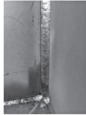
Fig.11 Intersection of hull member after welding
