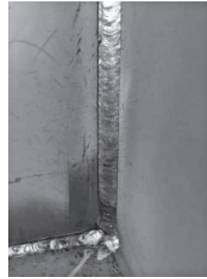
Fig.11 Intersection of hull member after welding
