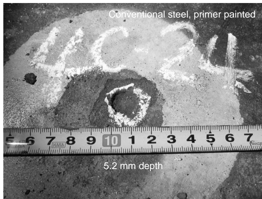
Figure 9: Typical example of pit on COT bottom plate (Ship B / 2.5 y).
