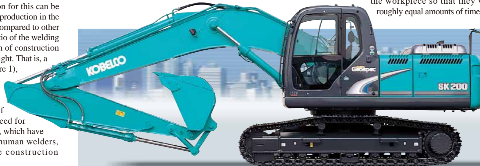
Figure 1: A20-MT class hydraulic excavator needs about 200kg of welding consumables to fabricate.
