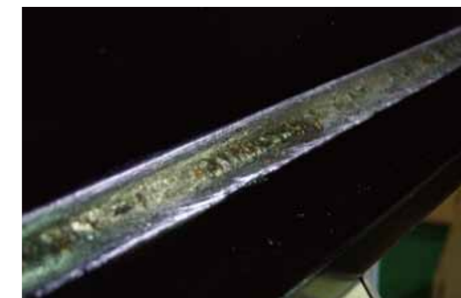
Figure 8: Weld bead appearance in tandem arc welding with a Dual-arc sensor.
