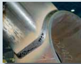
Vertical position weld appearance
