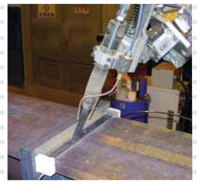
Automatic slag-removal device
