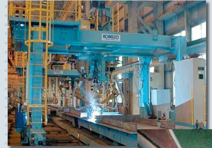
Twin Gantry Type System for Bridge Panel – ⑥
