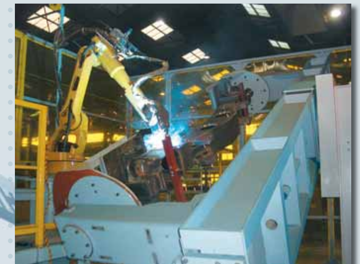
ARCMAN™ MP plus drop-axis two-motion-axis positioner (rotation and tilt)
