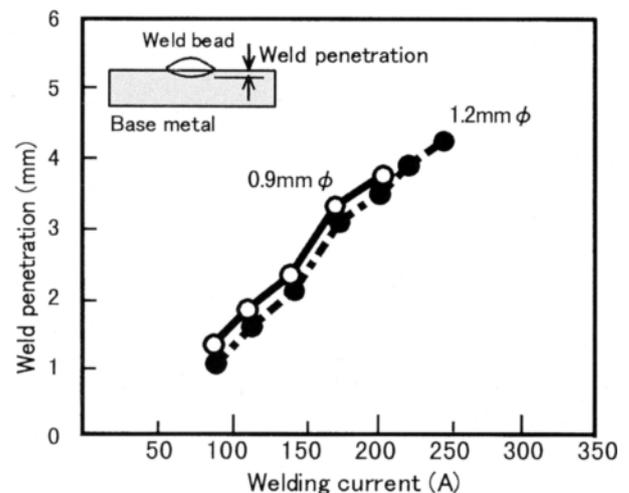
**Fig. 2 — Weld penetration of MG-51T as a function of welding currents with a short circuiting arc**
