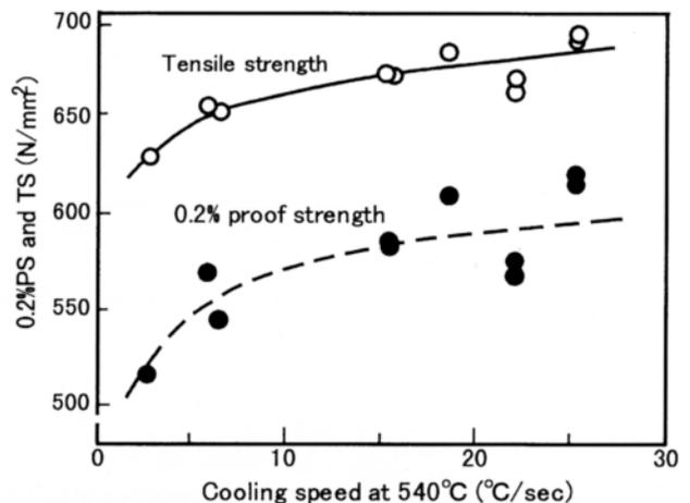
**Fig. 3 — Strength of LB-62L (4.0Ø) weld metal vs. cooling speed (As-weld; Power source: AC)**
