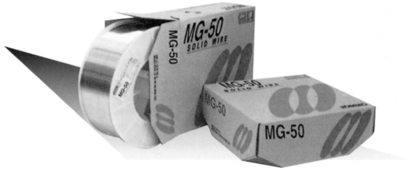
MG-50 is one of the most popular solid wires for gas metal arc welding of mid- and heavy-thick mild steel and 490N/mm<sup>2</sup>-class high strength steel with CO<sub>2</sub> shielding. Steel structures, construction machinery, and industrial machinery are typical applications of MG-50.
