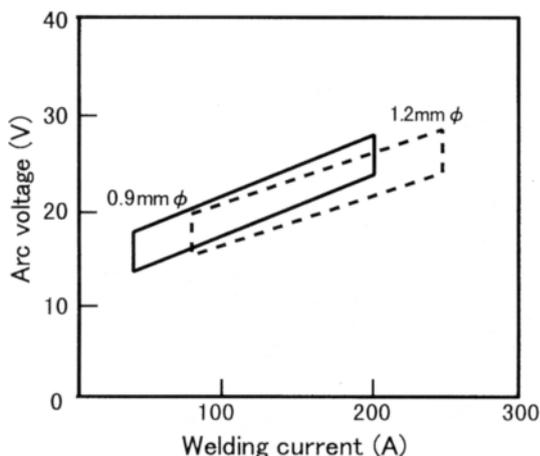
**Fig. 1 — Proper ranges of welding currents and arc voltage for MG-51T (0.9 mmØ, 1.2 mmØ)**
