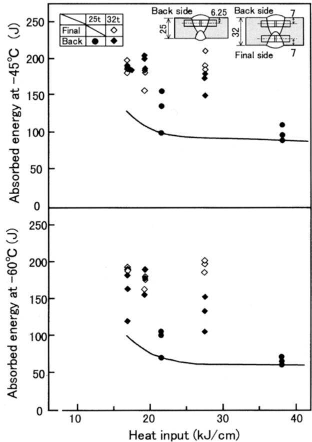
**Fig. 2 — Impact absorbed energies of LB-62L (4.0Ø) weld metal as a function of heat input in welding double-V groove joints in flat, horizontal and vertical-up positions. (As-weld; Power source: AC)**
