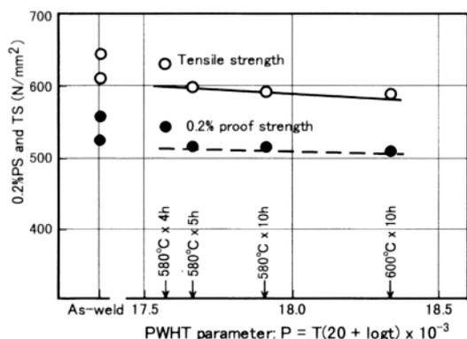
**Fig. 4 — Strength of LB-62L (5.0Ø) all-deposited metal vs. PWHT parameter (Power source: DC-EP, Heat input: av. 19 kJ/cm, Welding position: flat)**
