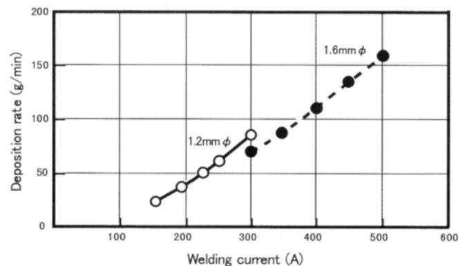
Fig. 2 — Deposition rates of MG-50 (wire extension: 15 mm for 1.2 mmØ; 20 mm for 1.6 mmØ)
