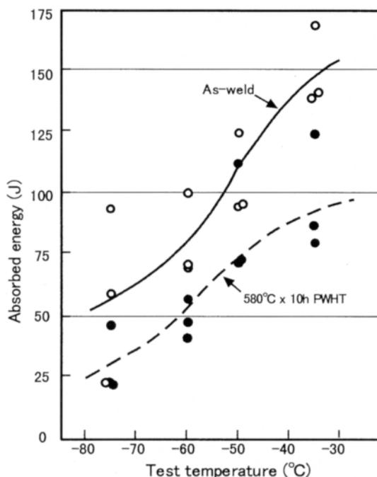
**Fig. 5 — The effect of postweld heat treatment on impact absorbed energy of LB-62L (4.0Ø) weld metal (Power source: DC-EP, Heat input: av. 38.7 kJ/cm, Welding position: Vertical up, Base metal: A537 Cl-2, Groove preparation: double V)**
