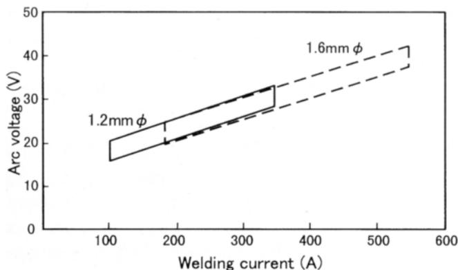
Fig. 1 — Proper ranges of welding currents and arc voltage for MG-50 (1.2 mmØ, 1.6 mmØ)
