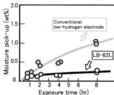
**Fig. 6 — Test results of LB-62L and a conventional low-hydrogen electrode on moisture pick-up under the controlled atmosphere: 30°C x 80%RH.**
