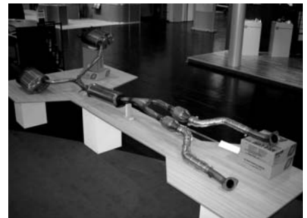
An automotive exhaust system flux-cored arc welded with MXA-430M
