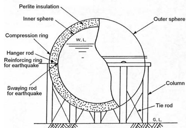
Figure 5: Cross sections over double-wall spherical tank.
