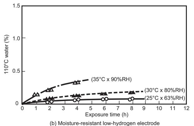
Figure 6: Moisture absorption curves of a moisture-resistant low-hydrogen electrode and a conventional low-hydrogen electrode tested under conditions of controlled temperature and relative humidity.
