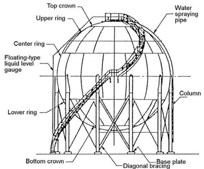
Figure 2: Spherical LPG storage tank.
