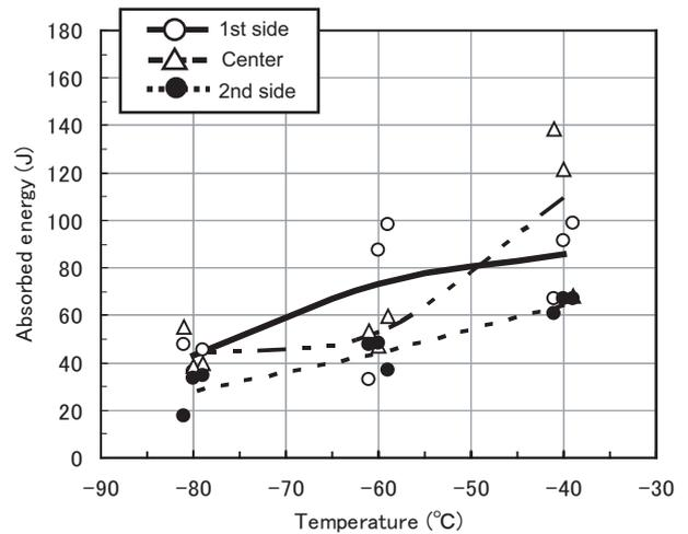
Figure 1: Charpy V-notch impact test results of a weld joint made with LB-7018-1 (3.2 and 4.0 mm $\varnothing$ ) and SM490A base metal (50-mm thick double-V groove) in the vertical position. (Heat input: 2.5-2.9 kJ/mm).
