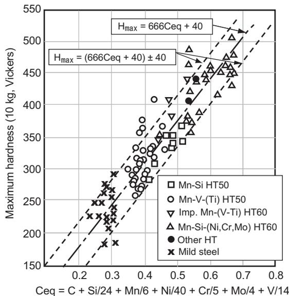
Figure 1: Maximum HAZ hardness vs. Ceq of 20-mm thick mild steel and high tensile strength steels (Bead-on-plate welding with a D5016 electrode) [Ref. 1].
