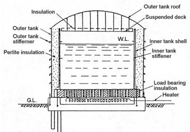
Figure 4: Cross sections over flat-bottom suspended-deck cylindrical tank.
