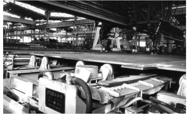
Figure 4: The FCB process achieved ultimate welding efficiency in one-sided submerged arc welding of hull plates.
