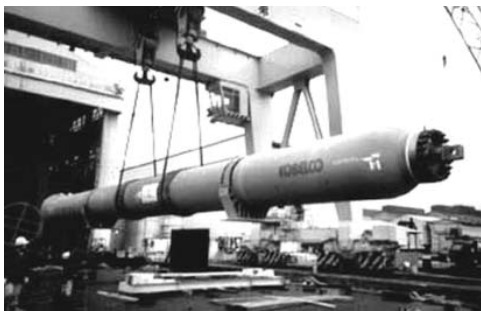
Figure 18: Kobe Steel fabricated the world's first state-of-the-art reactor vessel of 2.25Cr-1Mo-V-Cb-Ca steel in 1998 by using the matching welding consumables: CMA-106H , PF-500/US-521H , and TGS-2CMH .
