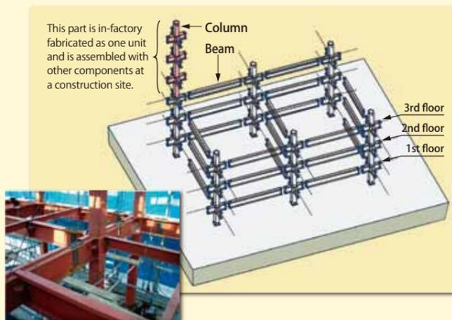
Due to the desire for large spaces in offices or factories, cold-rolled square or circular steel pipes, which do not require diagonal braces, have increasingly been replacing H-section steel columns. Indeed, square steel pipes or circular tubes are now applied in 95% of low and medium-rise structures. These columns and beams are constructed at the steel frame fabricator and transported to and assembled at the construction sites.
