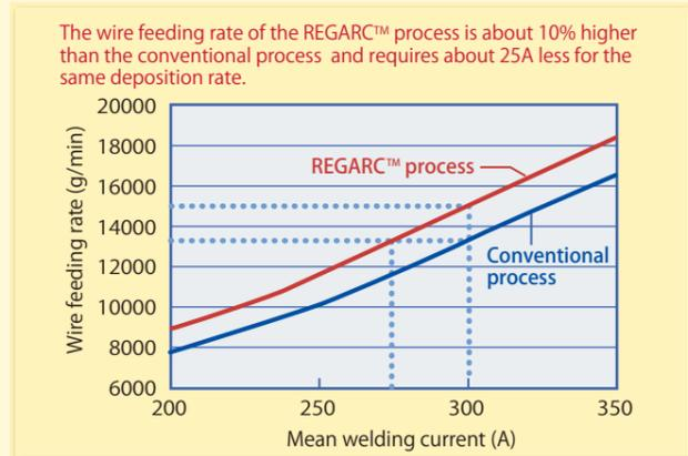
The wire feeding rate of the REGARC™ process is more than 10% higher than that of the conventional process. Because the pulsing welding current of the REGARC™ process is higher than that of the conventional process, resulting in higher Joule heat, the deposition rate (and overall
