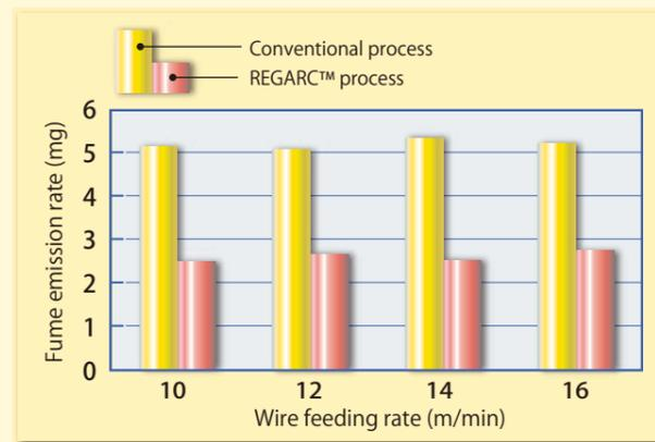
It is clear that the REGARC™ process generates nearly half the amount of fumes compared with the conventional process.
