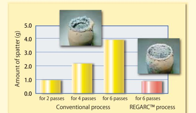
When spatter sticks to the inside of a nozzle, shielding may be reduced, resulting in poor mechanical properties as well as welding defects such as weld metal porosity. For this reason, robotic welding incorporates automatic nozzle cleaning and nozzle exchanging in order to maximize operation time.
