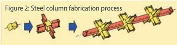
A section of a large column is fabricated by first welding the core part (left), then by welding the beams to the column joint (center) and finally by welding the column assembly (right).
