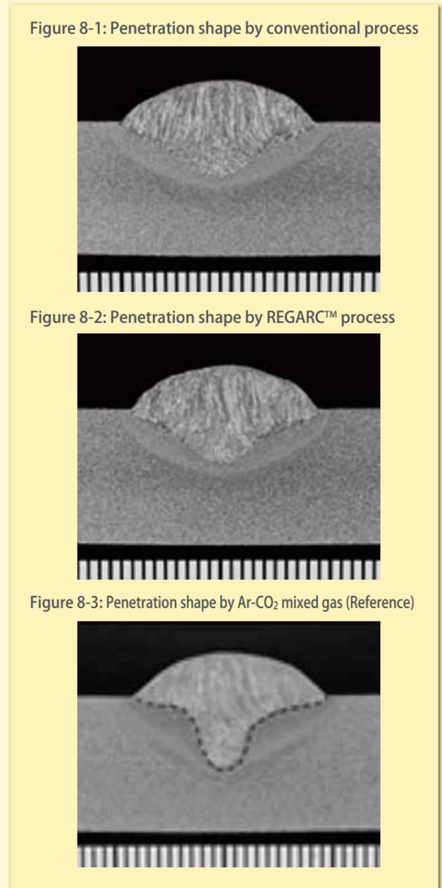
Even though the mean welding current of the REGARC™ process is lower than that of the conventional process, similar penetration is obtained (Figures 8-1 & 8-2) because of the higher peak current of the REGARC™ process. Hence, it can be seen that sound welding can be performed despite lower heat input.
