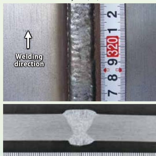
Note: 1. Welding position: Vertical upward (3G) 2. Current: 160A (DCEP)
