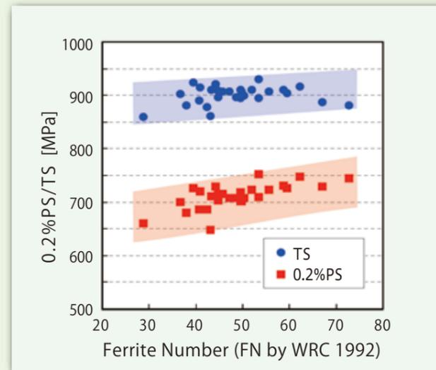
Figures 2 and 3 show the correlations between the ferrite number (FN), i.e. the ferrite content, and tensile strength/proof stress, and between the FN and notch toughness on the weld metal by the AWS E2594 type flux cored wire (FCW), respectively.
