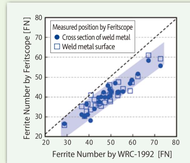
counting, which utilizes microstructures; referring to the Welding Research Council's (WRC)-1992 diagram composed of chemical compositions; or using a Feritscope, which applies eddy current and magnetic induction. At welding sites, the point counting method is seldom applied as it is difficult to handle. When FN control is necessary for butt joint welding, the Feritscope is preferred to determine pass/fail.
