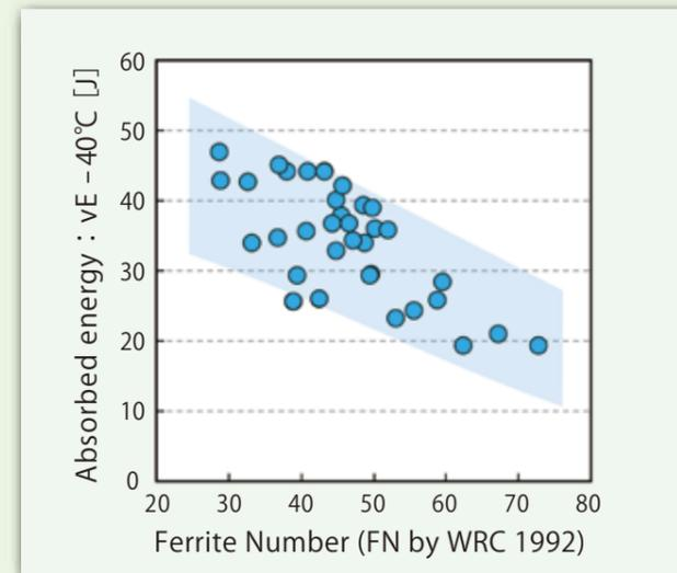
within a range from 30 to 65. In addition, because the weld metal is less corrosion resistant than the base metal, which is produced through a process of thermal refining, it is designed to hold slightly higher amounts of alloying elements (higher PREW) than the base metal. The Ni content of the weld metal is also designed to be higher than that of the base metal in order to optimize the ratio of austenitic and ferritic grains under as-welded conditions in many cases. (2),(3)
