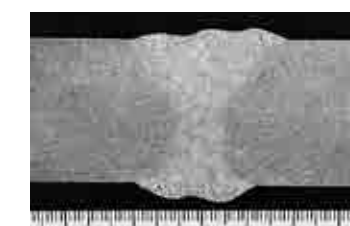
Figure 6: Macrostructure of MX-A410NiMo weld metal
