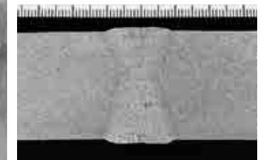
Figure 5: Macrostructure of DW-410NiMo weld metal
