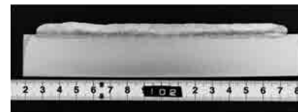
Figure 1: Macrostructure of DW-N625 overlay weld metal
