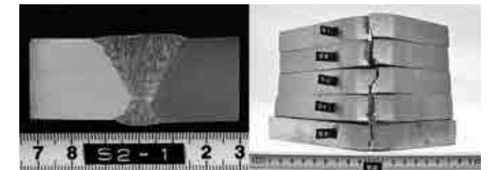
Figure 11: Macrostructure and side bend test results of a dissimilar joint welded by type 309
