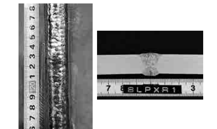
Figure 5: Bead appearance and macrostructure of DW-308LP-XR butt joint weld metal (3G upward position)
