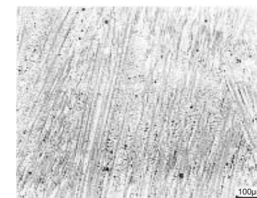
Figure 3: Microstructure of DW-NC276 all deposited metal in as-welded condition
