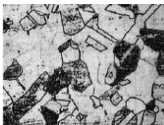
Figure 1: Microstructure of 304L type base metal (fully austenitic structure)
