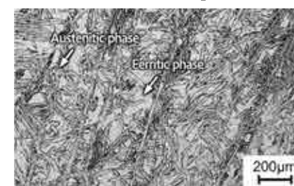
Photo 4: Microstructure of duplex stainless steel weld metal
