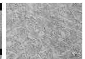
Figure 7: Microstructure of MX-A410NiMo weld metal
