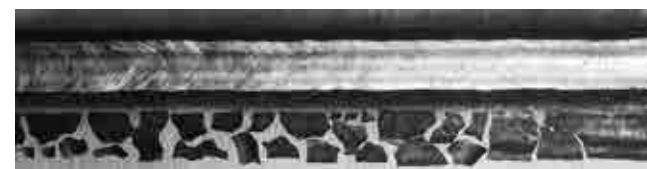
Figure 11: Bead appearance of DW-308L horizontal fillet welding by DW-308L
