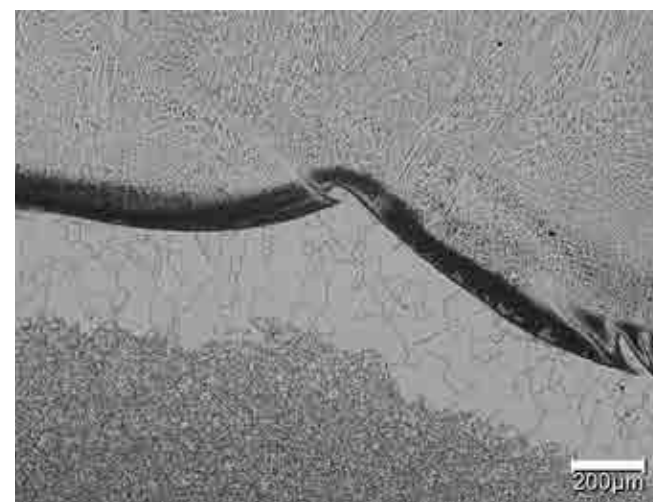
Figure 15: Decarburized and carburized layers after PWHT (710°C × 32 hrs) (Upper side: 309L weld metal; Bottom side: Base metal of 2.25Cr-1Mo steel)
