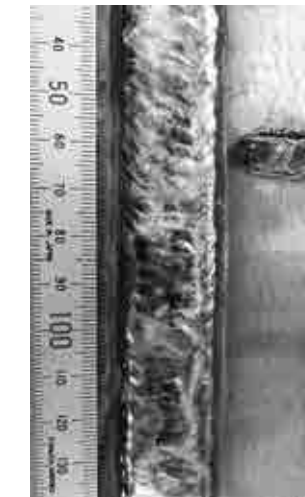
Figure 4: Bead appearance of DW-410NiMo
