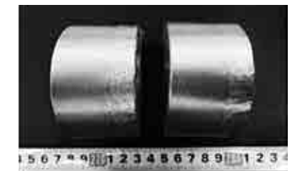
Figure 2: Side-bend test results of DW-N625
