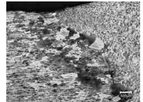
Figure 4: Grain growth in HAZ of ferritic stainless steel
