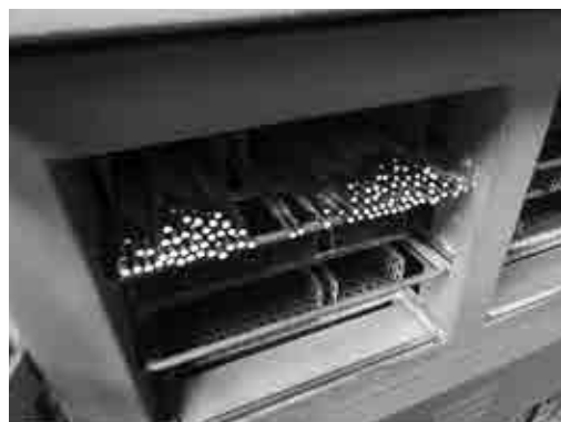
Figure 1: Oven for redrying electrodes
