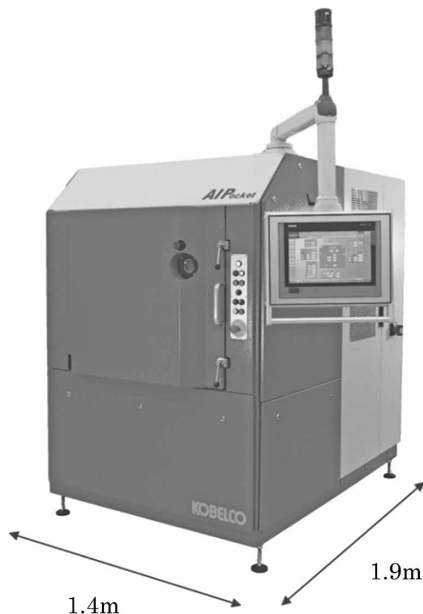
図7 小規模生産向け成膜装置 AIPocket™ の外観イメージ Fig.7 Schematic image of AIPocket™ system designed for small lot production batch
