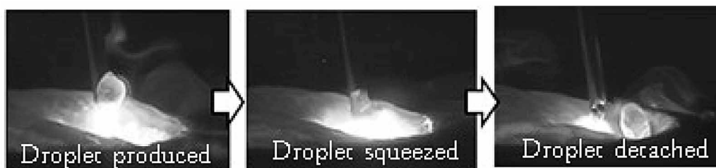
図6 New REGARC™プロセスの溶滴移行形態 Fig.6 Metal droplet transfer by new process
