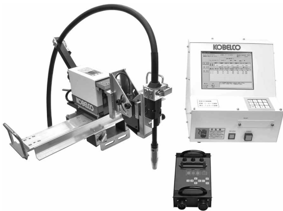
図1 小型可搬型Ni鋼用溶接ロボットKI-700外観 Fig.1 Appearance of KI-700 compact portable welding robot for nickel steel
