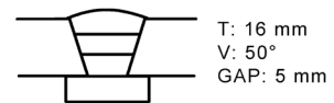
図14 突合せ継手の能率比較例 Fig.14 Efficiency comparison example of butt welding
