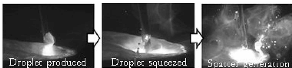
図5 REGARC™プロセスの溶滴移行形態 Fig.5 Metal droplet transfer by conventional process
