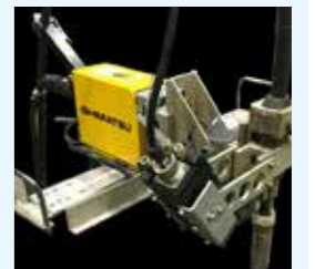
Compact and portable ISHIMATSU welding robot with visual sensor
