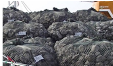
Submerged breakwater construction material (Filling material: Iron and steel slag hydrated matrix)
