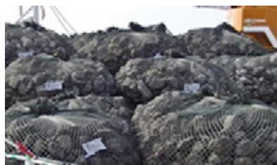
Submerged breakwater construction material (Filling material: Iron and steel slag hydrated matrix)
