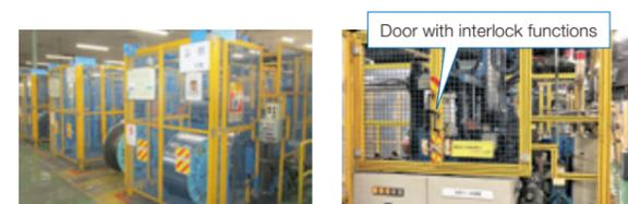
Safety fences with interlock functions have been installed to reduce the risk of unsafe access to rewinders and other moving sections of manufacturing processes at the Ibaraki Plant of the Welding Business
