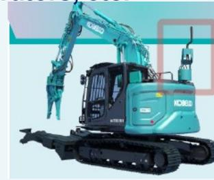
**Electric excavator (vehicle dismantling machinery)**
