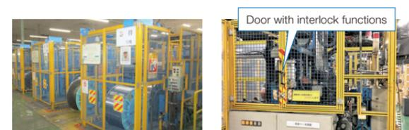
Safety fences with interlock functions have been installed to reduce the risk of unsafe access to rewinders and other moving sections of manufacturing processes at the Ibaraki Plant of the Welding Business
