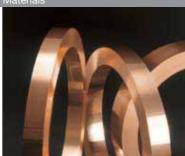
With circuits becoming more miniaturized and concentrated, we produce copper alloy products for high-strength, highly conductive semiconductor leadframes, terminals and connectors. Our superior reliability is supported by years of experience and firstclass technologies
