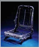
Kobe Steel's high strength steel sheet has enabled car manufactures to reduce the weight of cars and offer protection to drivers under crash conditions. The Company has commercialized in rapid succession an extensive lineup of high strength steel sheet.
