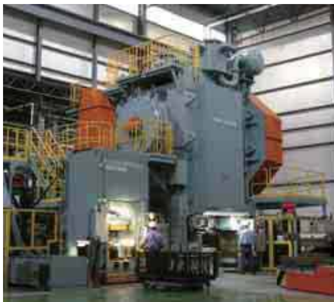
6,300-ton forging press at KAAP
