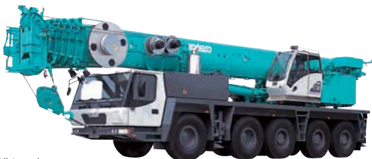
All terrain crane
