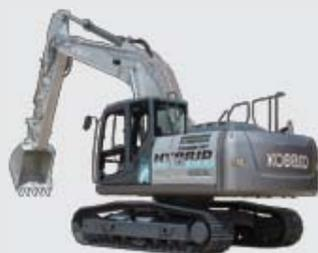
20-ton-class hybrid hydraulic excavator SK200H
