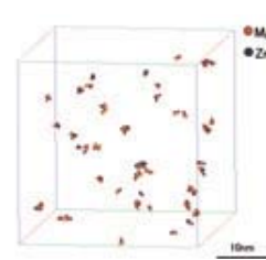
Cluster mapping of magnesium and zinc
