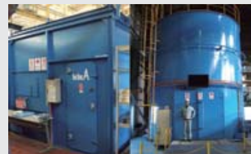
Cubic chamber (left) and domed chamber (right)
