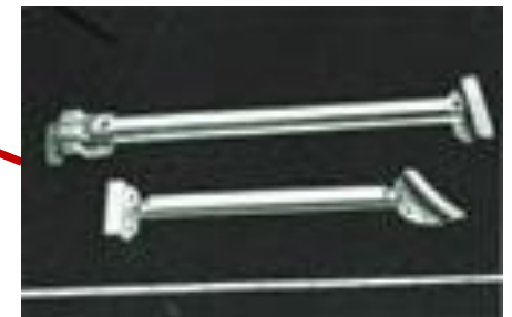
Door beams (with brackets)
